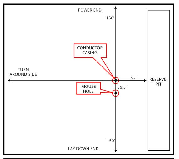
Note: <u>All</u> measurements are from the center of the conductor casing. The mouse hole is 86.5" from the center of the conductor casing w/ 0° slope (Angle). This rig has a top drive so the mouse hole should be a minimum of 75' deep (from ground level) with casing or liner with a minimum ID of 10". The reserve pit is a minimum of 60' from the center of conductor casing.
